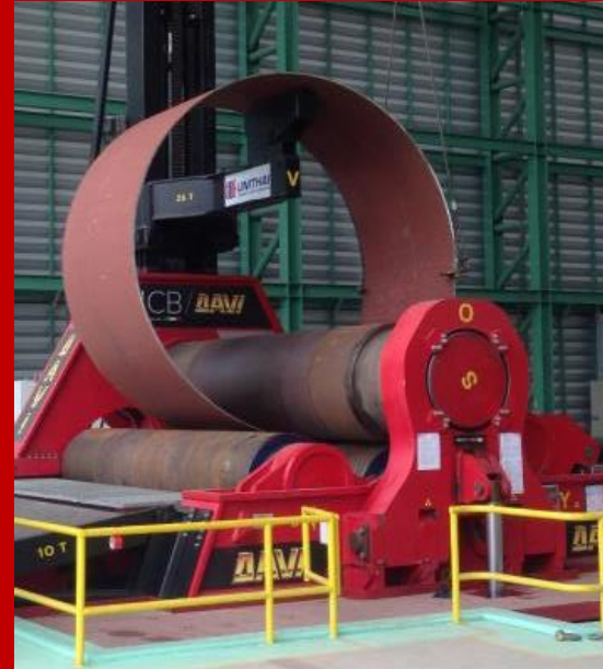
Plate Rolling Machine - 4 meter width, roll up to 135 mm. thick plate.
